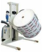
Toppy Webb Reels up to 1,000 kg Manual drive and electric drive Min and max reeldiameter 700-1.270 mm Grips the reel on the outside!
