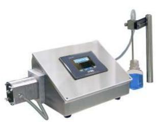
The HMI touch screen allows you to create, copy, and save text based recipes which dramatically reduces your set-up time as you switch between products, fill volumes, or container sizes because it is digitally controlled-no manual adjustments needed.
