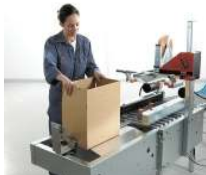
The case is held firm and is ready for filling.
