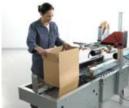
The case is led down on the rail and pulled back, and the bottom side flaps are folded
